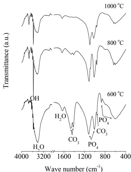
Fig. 1. FT-IR patterns of the apatite granules heat-treated at 600, 800, 1000 °C for 3 hours.
