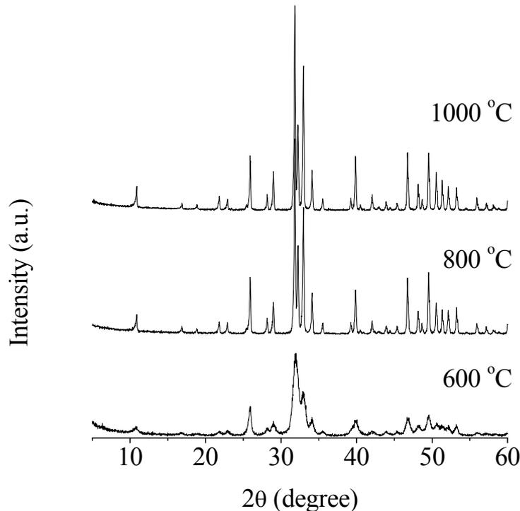
Fig. 2. XRD patterns of the apatite granules after the heat-treatment at 600, 800, and 1000 °C for 3 hours, respectively.
