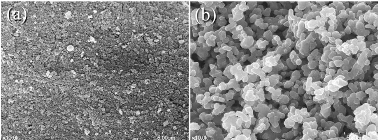
Fig. 3. FE-SEM photographs of the apatite granules heat-treated at (a) 600 °C and (b) 1000 °C for 3 hours.
